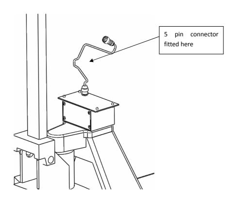
The Indicator bracket is fitted to the PTS using  $4 \times M4$  screws as the picture below shows, these should be tightened using the Allen Key supplied .
