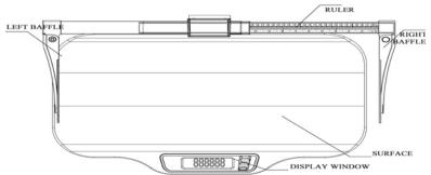
This scale has a maximum capacity of 44lb x 0.01lb (20kg x 5g) with a height range from 14 inches to 27.5 inches (35cm to 70cm).
