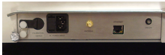
Wire seal preventing access to calibration switch
