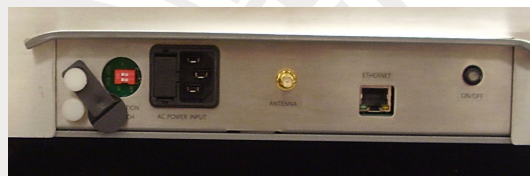
Cover open allowing access to calibration switch
