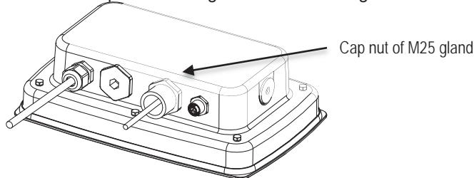
8. Warp the rubber seal onto Current Loop Output cable and Push it to the hole.
