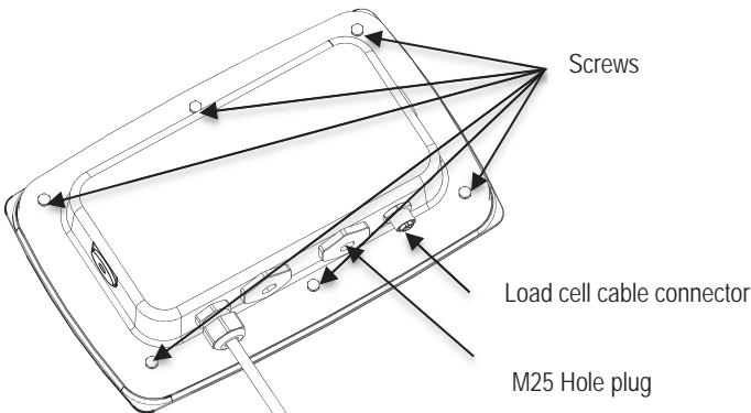
2. Rotate the rear housing down away from the front housing as shown.
