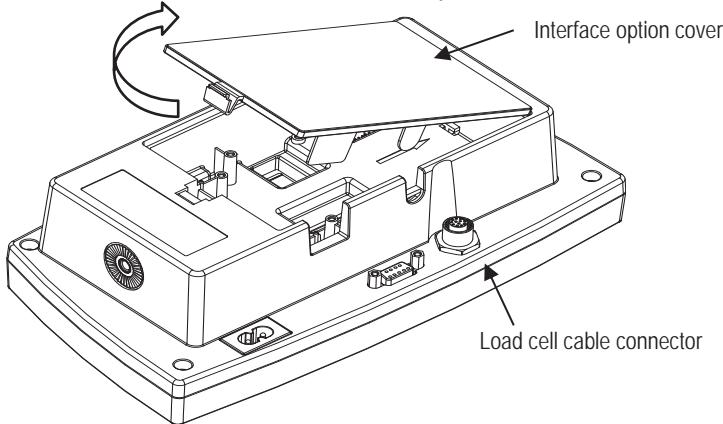
2. Break off the rib of the interface option cover as shown.
