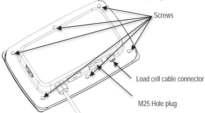
2. Take the rear housing down from the front housing as shown.
