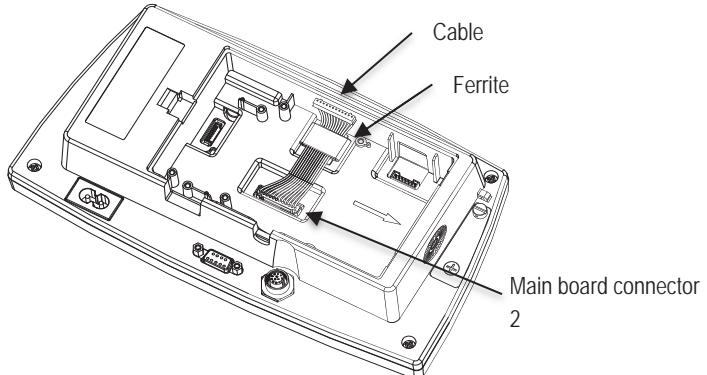
4. Install the Analog Current Loop board in the indicator using 2 screws as shown. Connect the 12 pin connector cable from the main board to the Analog Current Loop board 12 pin connector.
