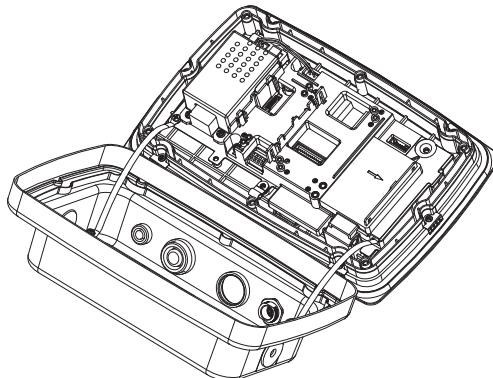
3. Connect the 12-pin Cable Connector included with the kit to the Main Board Connector 2. Place the ferrite in the slot of the black part as shown.
