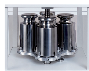
Positioners facilitating precise loading of weights
