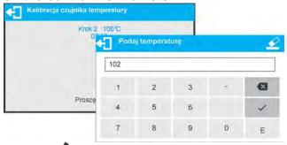
Press button to confirm, the third step of adjustment starts. The moisture analyzer halogen lamp starts to operate and the drying chamber is heated as long as necessary to provide specified temperature, which is next maintained for 8 minutes. After 8 minutes a numeric keyboard is displayed. Enter the moisture analyzer temperature that is displayed on the control thermometer.
