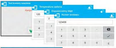
Enter testing temperature, maximum permissible error and the serial number of the temperature adjustment set.
