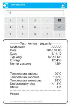
The temperature is maintained for 8 minutes (like for temperature adjustment procedure). After 8 minutes you shall see a window for entering temperature read from the installed adjustment set.
