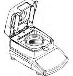
Load the weighing pan with the sample. Sample mass shall be selected on the basis of prior experience and tested material characteristics.
