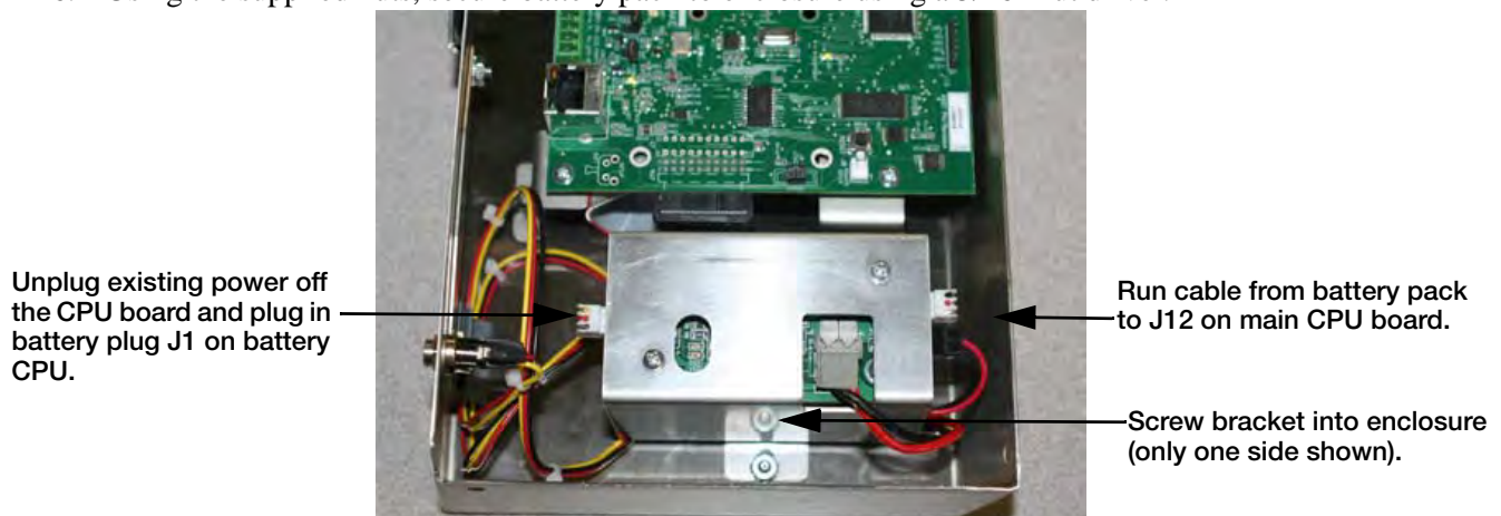
Figure 2-12. Secure Battery Pack into Enclosure
