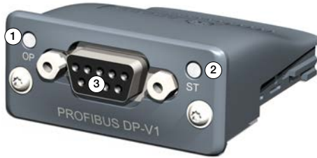
Figure 2-6. PROFIBUS DP Status LED Module
