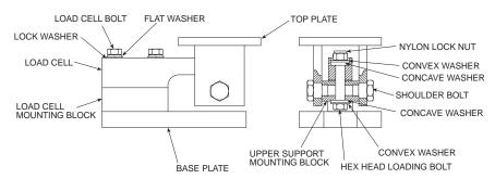
The type of installation, structure of the vessel supports, and strength of the mounting surface determines the method of locating, attaching, and assembling the RL1900 Mounting Assembly. Carefully consider three areas that commonly cause accuracy problems:
