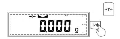
2. When weighing, always place the mass in the middle of the pan. The weighed result may be taken when the stabilization indicator appears on the display.
