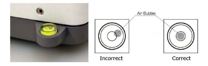
4. After leveling the scale, you may plug the AC adaptor to the AC adaptor socket located in the rear of the scale.
