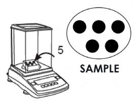
4. The weight of the sample will be displayed as it is placed on the pan. Once the weight of the sample stabilizes and the stability indicator appears on the display, press the MENU key to enter the main menu.
