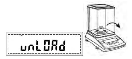
10. Once the weight is removed, the scale will continue with calibration adjustment. "WAIT" will be displayed during the remainder of the adjustment process. Once finished, the scale will automatically return to the weighing mode.
