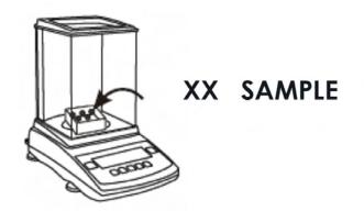
3. The weight of the sample will be displayed as it is placed on the pan. Once the weight of the sample stabilizes and the stability indicator appears on the display, press the MENU key to enter the main menu.
