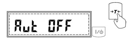
Note: AZSM is automatically enabled for 10 minutes after the scale is turned ON, regardless of its ON/OFF configuration.
