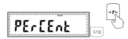
5. Commands "PER OFF" and "PER ON" will be displayed sequentially. To proceed with percent weighing and set the reference sample weight, press the T key when command "PER ON" is displayed.
