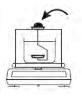
10. Once the weight of the object stabilizes, press the P key. Command "M1" will be displayed indicating that the weight of the object in air has been stored in the formula.
