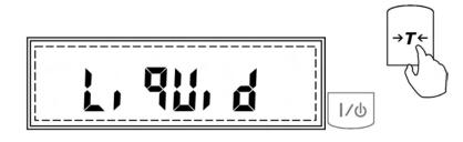
6. Once LIQUID is selected, command "PLUNGER" will be displayed, indicating to enter the volume of the plunger used in the density kit, which can be found on the plunger hook included with the density kit.
