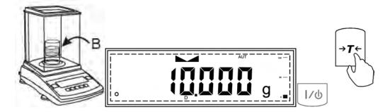
10. To check the total weight of the ingredients at any time, press the FUNCTION key. The SUM indicator and the total weight of the ingredients in the container will appear on the display. To clear the total, press the T key when the SUM indicator is displayed. To return to totalizing and add more ingredients, press the FUNCTION key once again.
