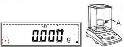
7. Once the weight of the ingredient stabilizes and the stability indicator appears on the display, press the T key.
