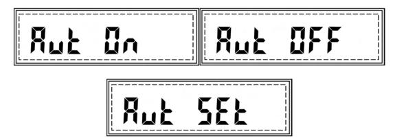
4. To enable AZSM, press the T key when AUT ON is displayed.
