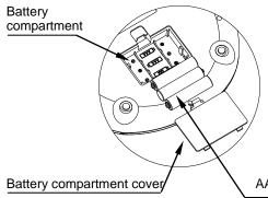
Remove the battery compartment cover and insert three batteries(AAA size) into the battery compartment, taking extreme care that the polarities plus and minus is observed.
